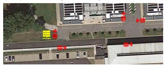
Figure 3: Layout of the cooperative traffic lights and the road side unit installed at JRC Ispra by Swarco Mizar.
