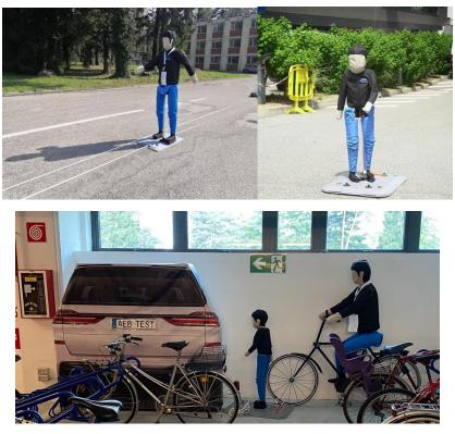
Figure 4: Example of targets used for vehicle safety testing.
