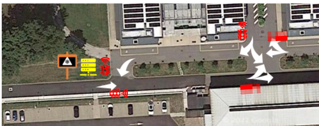
Figure 3: Layout of the cooperative traffic lights, the road side unit and the variable message sign installed at JRC Ispra by Swarco Mizar.
