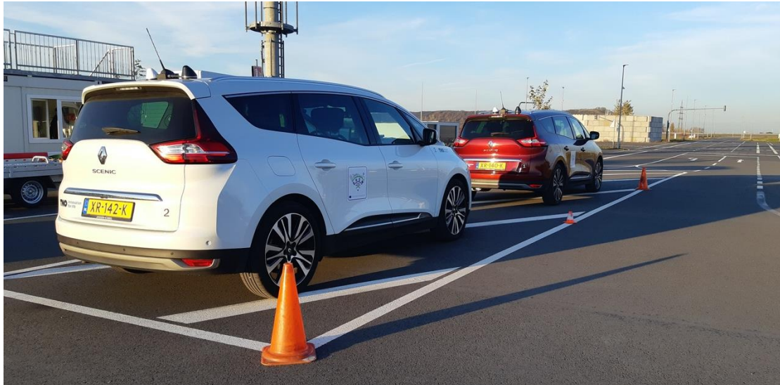
Figure 21: Retrofitted level 3 automated vehicles at the Brainport validation site
