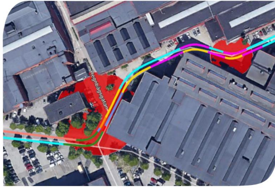
Figure 12: Zone 4, areas where the GNSS signal is not reliable.
