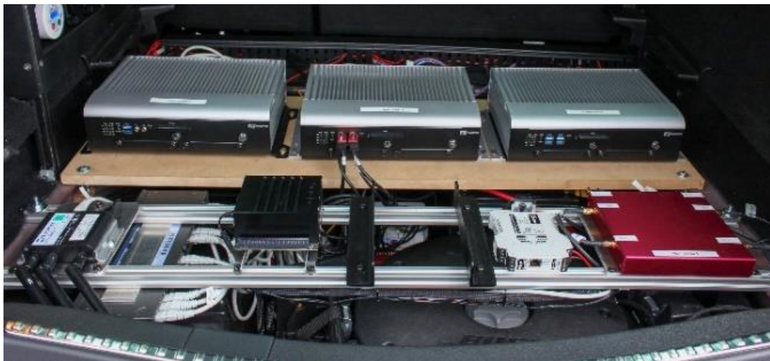
Figure 22: Sensor, communication and processing platforms located in the trunk of the TNO carlabs
