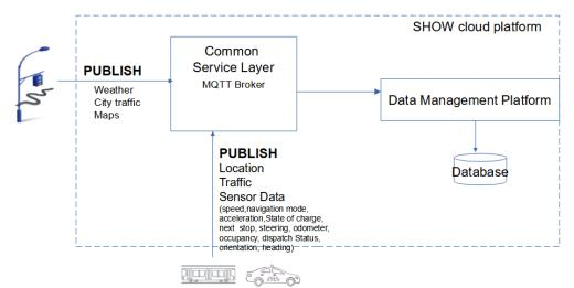
Figure 23: MQTT APIs for ETA service
