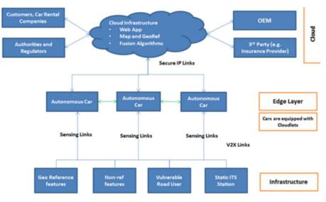
Figure 6: Platform Architecture for AVs [12].
