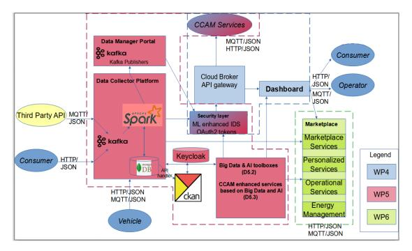
Figure 19: Inter-component relations of Data Portal and Big Data collection platform and their connection to SHOW web-services (source D5.1 [14]).
