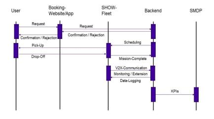
Figure 5: Example of service information flow diagram (UML sequence diagram)
