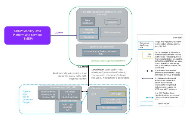
Figure 13: Functional architecture diagram – focus on the LFMP (EasyMile Local Supervision Platform)
