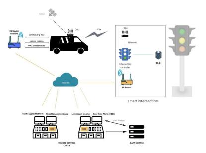
Figure 33: Components of the local architecture
