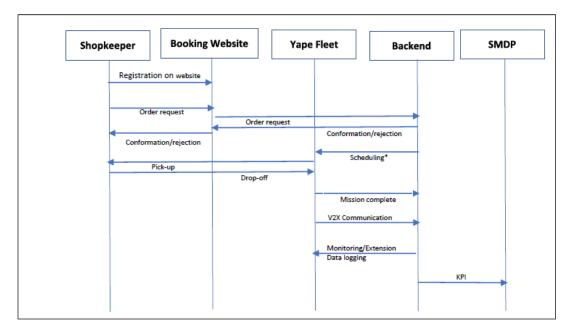
**Figure 36: Logistics service information flow** (\*During scheduling, MapPoint of the shop is selected and Yape fleet automatically selects the shortest path (in predefined Yape path) from control room to the shopkeeper)
