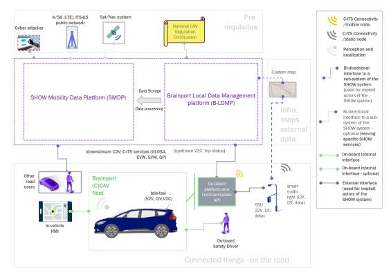
Figure 31: Local actors diagram for Brainport pilot site Table 9: Local actors' role and connectivity enabled (when applicable)
