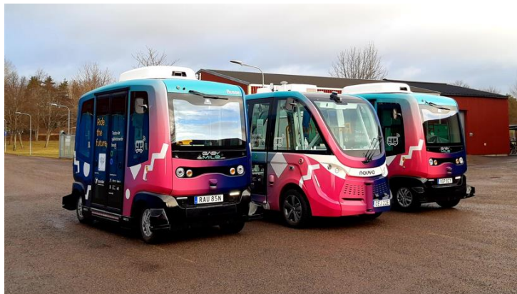
Figure 75: The three AV shuttles in Linköping. The middle shuttle is a Navya DL4 Arma, the two on the sides are EasyMile EZ10 Gen2. Photo My Weidel, VTI.
