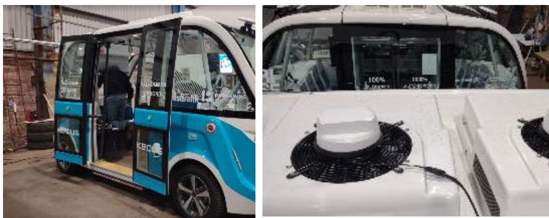
Figure 53: Left: Navya shuttle at site Lindholmen/Gothenburg with GPS antenna – Right: 5G vehicle antennas on the roof of the Navya shuttles.
