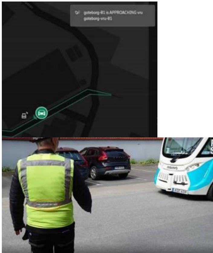
Figure 59: Vehicle-VRU geofence overlap trigger notification messages and audio-visual messages at VRU sensor and in the SHOW Dashboard.
