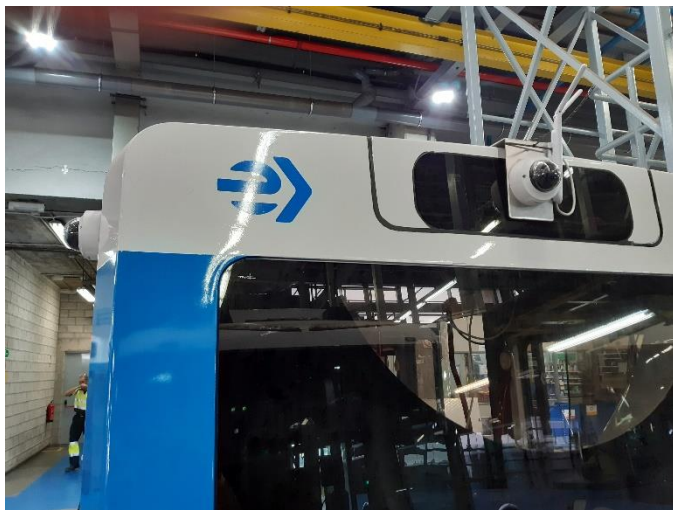
Figure 134: Madrid Mega pilot: UC1.7 specific cameras and WiFi antennas installed on Gulliver.
