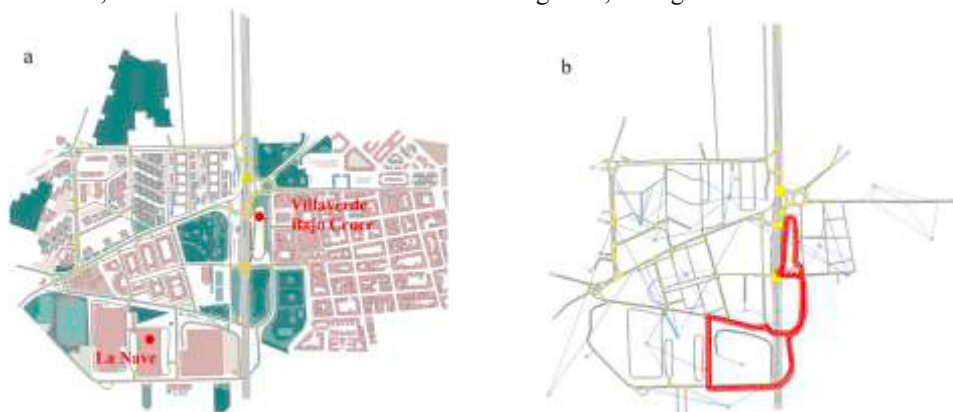
Fig. 1. Villaverde network in Aimsun Software and the shuttle service: (a) two connecting points; (b) circular route.
