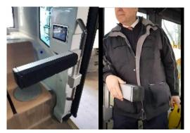
Figure 20: Safety arm for incidents' avoidance - Linköping (source: My Weidel/VTI)
