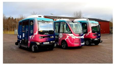
Figure 7: The three AV shuttles in Linköping. The middle shuttle is a Navya DL4 Arma, the two on the sides are EasyMile EZ10 Gen2 (source: My Weidel/VTI)
