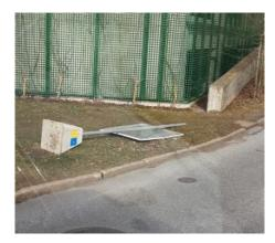
Figure 57: LiDAR markers were put down by strong winds (source: Keolis)
